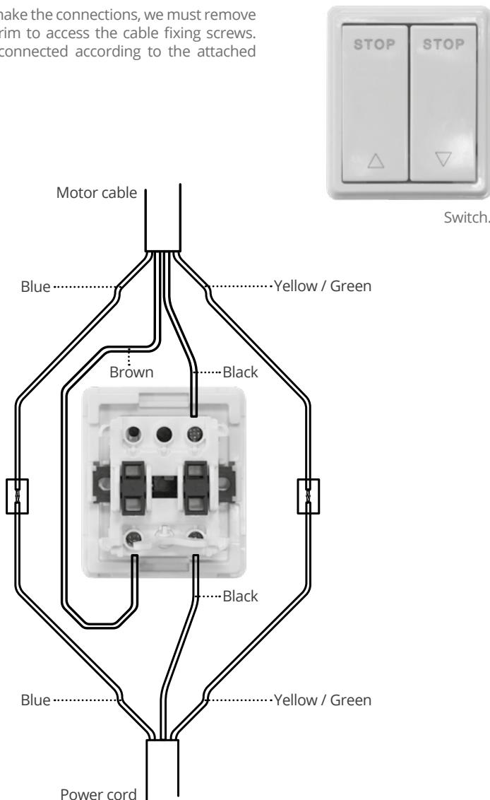
Once the motor connections have been made with the switch, the switch cover must be placed and the switch fixed in a fixed and protected place. The connections of the connections must be correctly installed and secure for a correct use of the awning motor.
