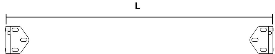
2. Present the arm brackets on the wall, mark and drill to fix them in place.
